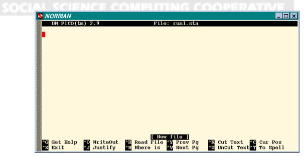
The status line at the top of the display shows PICO's version, the current file being edited and whether or not there are outstanding modifications that have not been saved. The third line from the bottom is used to report informational messages and for additional command input. The bottom two lines list the available editing commands. You simply enter text to begin your editing session. Each character typed is inserted into the buffer at the current cursor position.
